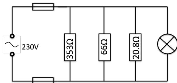
d)  $I = U/R = 230V/20.8\Omega = 11.05769 \text{ A} = 11.1 \text{ A}$  (3 signifikante Ziffern)
